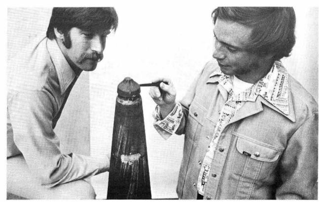
RECOVERED NOSETIP, no longer hemispherical, is focus of Ralph Clark's and Ed English's attention. Streaks are aluminum melted by heat generated at the tip.
